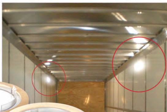
Photo illustrates Truck-Lite Sky-Lite's installed into traditional trailer walls.
