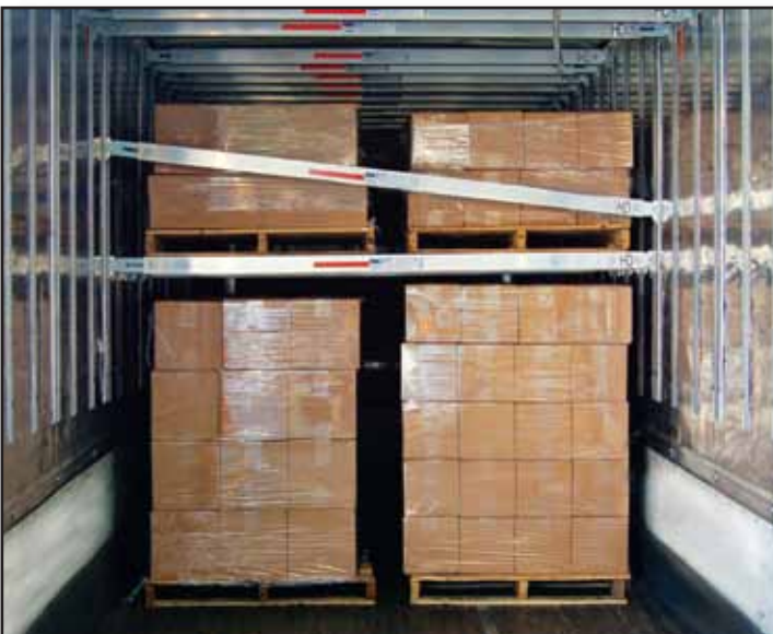
✓ Use Beam to Secure Pallets
